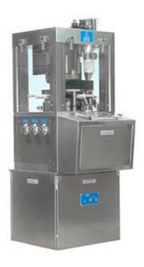
ZPS-8 rotary tablet press is a kind of intelligent small rotary tablet press. It is suitable for small batch production of pharmaceutical industry R & D centers and laboratories.
