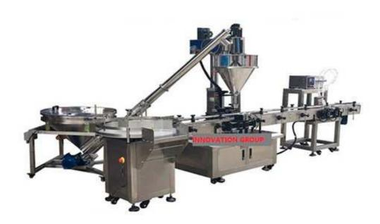
The automatic powder filling line includes: semi-automatic bottle unscrambler  $\rightarrow$  automatic feeding machine  $\rightarrow$  single-head powder filling machine  $\rightarrow$  magnetic pump filling. The assembly line configuration can be selected according to the requirements of the product;
