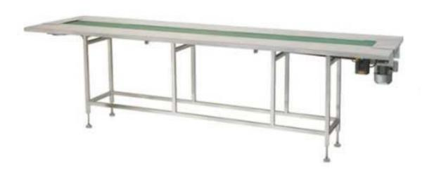
The Packing conveyor belt is having stainless steel Table Top with moving Endless sandwich belt in the center. Tabletop is fixed to the same structure made out of SS 304 square pipe & supported on adjustable bolts. Tabletop is of 12 inches working space on both side of the conveyor belt for final visual inspection & packing into the box.
