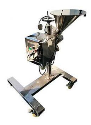
The machine is widely applied in such industries as medicine, chemical industry and food, achieving good effect. With reasonably designed filter screen and rod, the machine can crush a pile of friable materials. According to the centrifugal force principle, it uses filter screen with special pores to carry out careful sieving. The special fiction filter screen rod can crush solid particles and grind large agglomerates.
