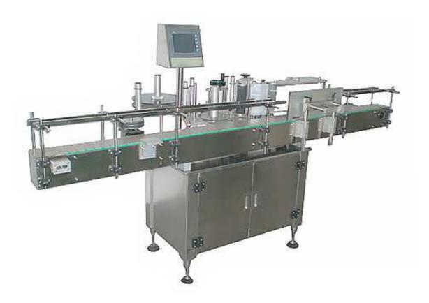
The labeling machine is specialized in round bottles. When labeling, the bottle will automatically rotate to allow the labeling device to apply the pressure for labeling.
