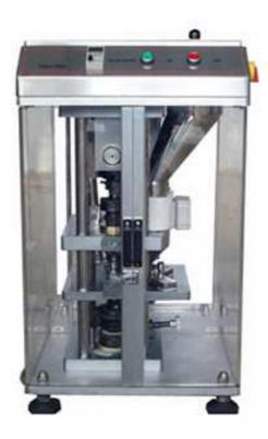
Developed through the absorption of the international advanced technologies, this machine can press round or irregular tablets from various granular materials. It is applicable to trial manufacture or small scale production in lab, hospital and Science research institutes etc.
