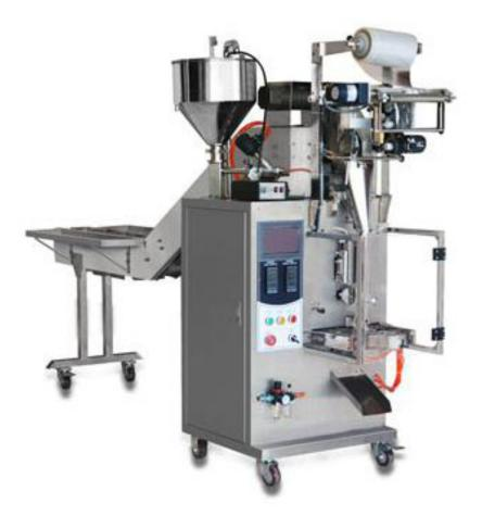
The MK-60HY vertical form fill seal machine realizes the synchronous packaging of irregular materials and liquids through the in feed conveyor and liquid filler. It helps to effectively package materials that are difficult to handle automatically. For example, the packaging of medical alcohol cotton balls is realized by feeding alcohol with liquid filler and feeding the cotton ball manually through the infeed conveyor.
