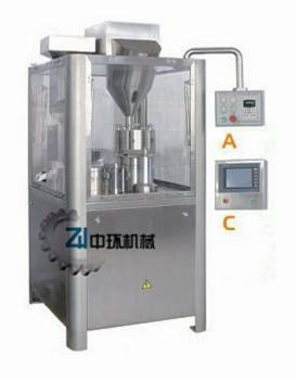
This automatic capsule filling machine is adopted with plugs filling, intermittent operation and frequency conversion speed adjustment. It's suitable for automatically completing feeding capsules, separate capsules, filling capsules, closing capsules (waste capsules rejection) and finishing products with capsules in powder and pellets.
