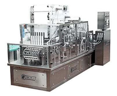
**Performance:** Servo Driven Fully Automatic Linear Filling and Sealing machine for Filling, Sealing & Capping of Pre-Formed Containers
