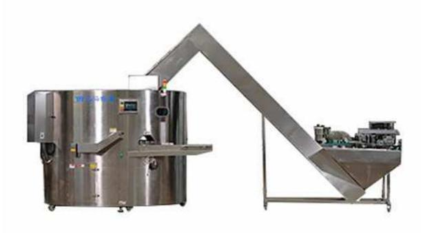
This machine adopts advanced technology, PIC intelligent control, and this machine does not change the mould can arrange for size similar and different shape plastic bottle, could use detergent square bottle or bottle with handle, and such as shampoo bottles, soy plastic bottles.
