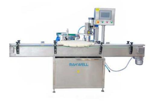
Automatic liquid filling machine is a high-tech product researched and developed by our company. It is suitable for products of liquid such as oral liquid, e-liquid, eye drop etc. It is widely applied for filling of products in such industries as food, cosmetics, medicine, grease, daily chemical industry, detergent, pesticide and chemical industry etc.
