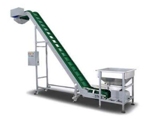
Inclined PVC belt conveyor is well suitable for the free-flowing products in the food, agriculture, cosmetic and chemical industry.
