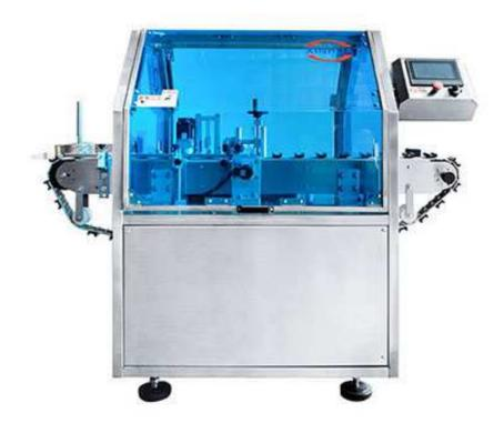
The lipstick shrink sleeve labeling position can be top and bottom sleeve wrapping, cap sleeve wrapping, or partial sleeve wrapping. Any place that customer wants to put the shrink sleeve on the stick. And XINHUA also provide automatic line solution which includes automatic lipstick feeding device, sleeve applicator, heat shrink tunnel, inspection machine and box packing machine.
