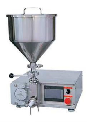
This filling machine uses peristaltic pump, most suitable for small volume products. Filling precision is extremely high. Sanitary benefits of using silicone filling tube are easy cleaning, able to replacing old tubes at any time, avoiding cross contamination for filling different liquids. 4.3" color touch screen is convenient to enter filling volume directly.
