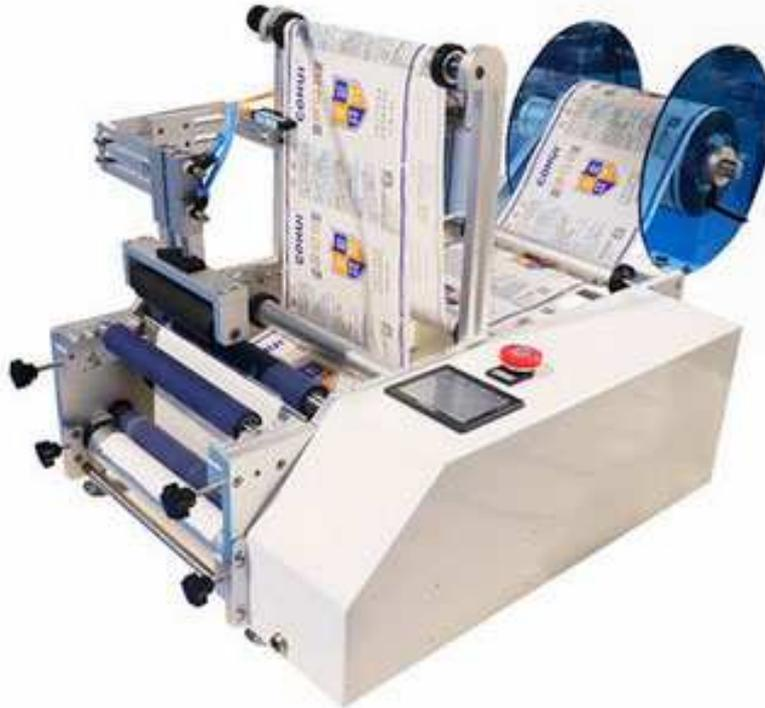
It is suitable for all kinds of cylindrical objects and small taper round bottles, such as xylitol bottles, cosmetic round bottles and wine bottles. It can realize full cycle/half cycle labeling, circumferential positive back labeling, and the distance between positive and negative labels can be adjusted arbitrarily.
