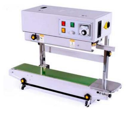
Plastic bag sealing machine is a machine to seal the container filled with packaging, after the product is loaded into the packaging container, in order to make the product sealed and preserved, maintain the quality of the product, to avoid the loss of the product, it is necessary to seal the packaging container, this operation is completed on the sealing machine.
