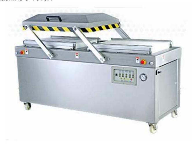
Heavy Duty Double Chambers Vacuum Packaging Machine from Jaw Feng Machinery Co., Ltd. is made of stainless steel, in line with food hygiene and safety. Wheels are with brake. Waterproof digital display panel. Programmable for data up to 10 set-ups. Each gum chambers configuration permits alternative operations for one operator
