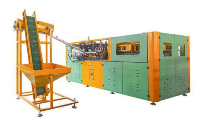
Full automatic blow molding machine is suitable for producing PET plastic containers and bottles in all shapes. It is widely used to produce the carbonated bottle, mineral water, pesticide bottle oil bottle cosmetics, wide-mouth bottle and hot fill bottle etc.
