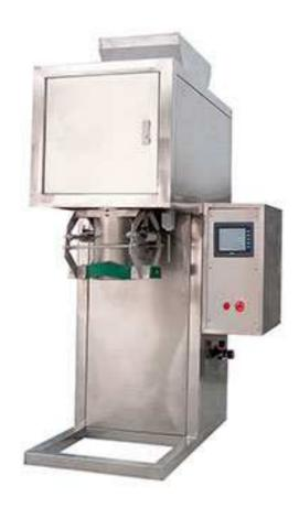
10kg Dry Powder Net Weigh Auger Filler is my a new generation of intelligent electronic weighing packaging machine developed by our company. With a reasonable structure, stable running, easy operation, high weighing accuracy characteristics.
