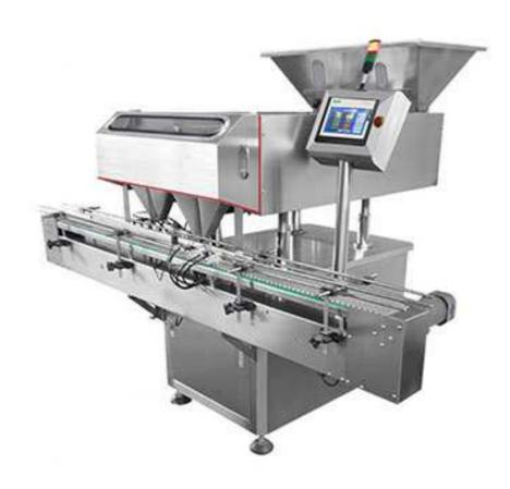
RQ-DSL-32 Gummy bear counting and bottling machine produced by Guangdong Rich Packing Machinery Co.,Ltd adopts the most advanced vibration multi-channel blanking method in the world and is designed according to GMP standards.
