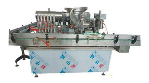
This jam filling and sealing machine is the main part of jam production line, and it is mainly used for filling, capping, and sealing 30-500ml bottles.
