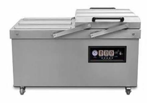
DZ-600/4SC floor type double chamber vacuum packaging machine for small bag vacuum packing. The double chamber vacuum packaging machine can seal different types bags with different thickness such as aluminum foil bag and transparent vacuum bag (nylon). It has double vacuum chamber working in turn, and the seal time and vacuum time can be adjusted sepeartely. It has four seal bars 600mm length each chamber.
