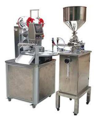
Automatic plastic cup filling and sealing machine is pneumatic type rotary sealing machine, suit for sealing PP/PET/PS/PVC..., rectangular, square or round kinds tray/cup, possible add with filler, conveyor.
