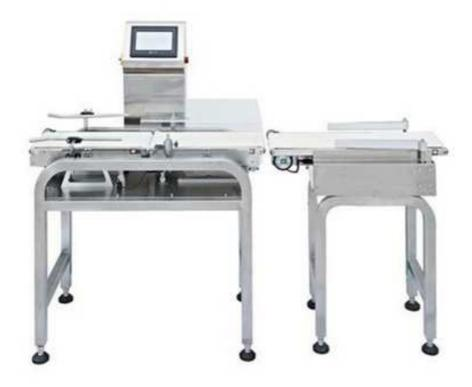
Standard Check Weigher can handle various packaging forms, including bulk paper bags, plastic bags, cartons, metal film packaging and so on. The maximum conveying speed is 55 m/min.
