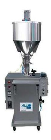
This Mixing Filling Machine is suitable to measurably fill the ointment materials with high viscosity and poor flow ability. The hopper is equipped with a frame mixing system. The machine is easy to clean and operate, conforming to GMP standards.
