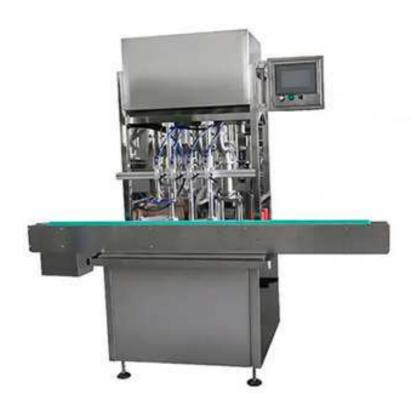
The filling machine is specially made for liquid with paste such as tomato paste, honey, jam, gel, peanut butter, oil etc. The automatic honey filling machine adopts Japanese Mitsubishi PLC program system to control. The machine adopts piston pump and for filling. By adjusting the position pump, it can fill all of the bottles in one filling machine, with quick speed and high precision.
