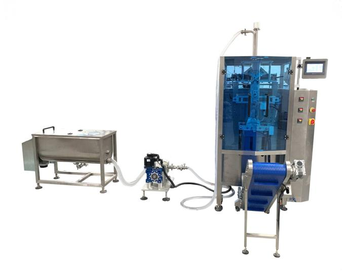
Automatic butter sauce packing machine includes servo rotor pump and reciprocating technology packing machine; Because the sauce has seeds and sesame which cannot be filled well by common liquid pump and reciprocating machine can work more stable.
