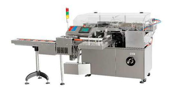
This series packing machine could adopt many feeding ways, could feed the product by manual, and also could connect with different model of boxing machine.
