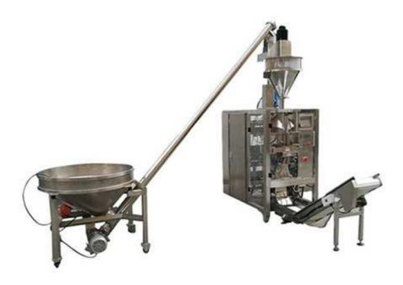
The Automatic Stick Powder Packing Machine uses advanced PLC control system, bilingual display in Chinese and English. The packaging speed and the length of the bag can be adjusted steplessly within a certain range without replacing parts. The double synchronous belt is used to pull the film, the cylinder is controlled to be tensioned, the automatic correction is performed, and the automatic alarm protection function is adopted to greatly reduce the loss.
