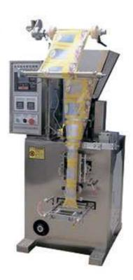
DXDF-350 powder automatic packaging machine is suitable for medium bag powder automatic packing. This equipment is mainly applicable to the packing of milk powder, sesame paste, strong bone powder, spices, Ganoderma lucidum powder, granules and other items.
