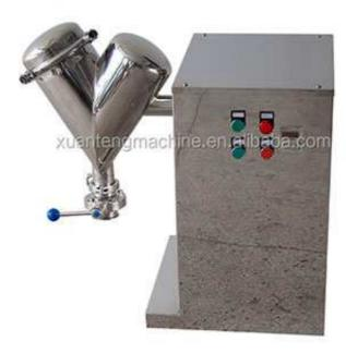
This machine is mainly used in pharmaceutical, chemical, electronic, food and other industries for powder, granule and other materials uniform mixing. Structural Features: This machine is mainly composed of mixing cylinder, frame, transmission system, electrical system and other parts, it is the use of two asymmetric cylinder, gravity mixing, the material in the cylinder continuous accumulation, continuous dispersion, generally after about 5-15 minutes of mixing.
