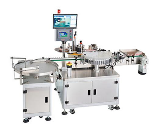
Suitable for high speed, high precision vertical labeling application of stably standing cylinder containers in various industries, and capable of labeling full or half round. Star wheel driven has two driving modes: continuous and intermittent type, suitable for pharmacy, daily products, chemicals, food, beverages, etc.
