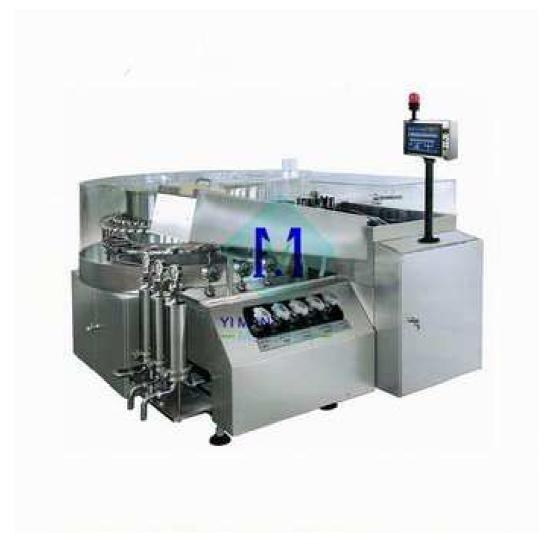
The Vertical Ultrasonic Washing Machine is used for washing bottles and containers. It performs the following procedures automatically: bottle conveying, ultrasonic washing, rinsing with air-water alternatively, and bottle outputting.
