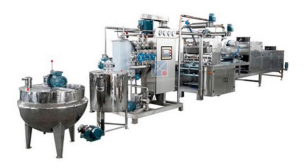
SGD150/300/450/600 servo driven PLC controlled automatic hard candy depositing machine is the most advanced production line for deposited hard candy and lollipop manufacturing. This line mainly consists of auto weighing and mixing system (optional), pressure dissolving system, microfilm cooker, depositor and cooling tunnel and adopt the advanced servo system to control the processing. Besides, this line also has following characteristics:
