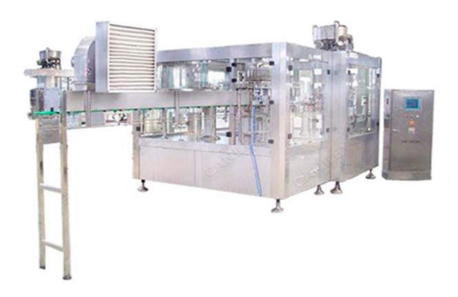
The complete set of juice filling packaging line is designed to fill juice and beverage into bottles. The automatic juice filling line integrates filling, capping and labeling in one. It is mainly aimed at the hot-filling production of plastic bottle juice beverages. The filling is stable and accurate, ensuring the material filling temperature and reducing material loss
