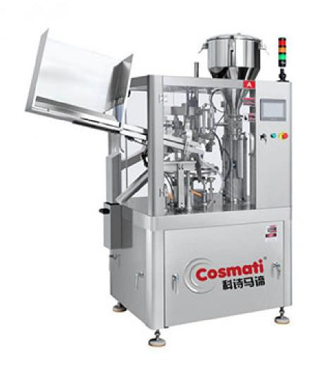
This equipment has a high degree of automation, automatic tube loading, automatic color marking, automatic tail sealing, batch number printing, and automatic tube discharge. Using the internal heating method, use the Swiss-made "LEISTER" air heater to blow hot air from the inner wall of the tube to melt the plastic.
