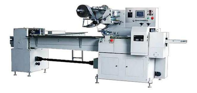
This machine is (a)on-edge auto packer, which can realize scattered pieces aggregate packing without tray. Application (It can be applied) to Biscuit, Snow pastry, chocolate, Table and Soap etc. which has regular shape goods, widely used in food processing pharmaceutical and chemical engineering.
