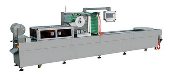
Full-automatic thermoforming vacuum packaging machine is suitable for various kinds of food, such as fish tofu, single piece of bean curd, double pieces of bean curd, areca-nut, spicy food, pickles, chilled mea etc.
