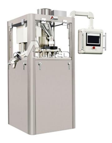
Rotary tablet press fully complies with GMP pharmaceutical requirements. It is a continuous automatic rotary tablet press that compresses powder and granular raw materials into tablets in pharmaceutical, chemical, electronic, food, laboratory and other industries. The main working process is divided into: filling; tableting; outputting. The Filling and tableting with adjustment control mechanism.
