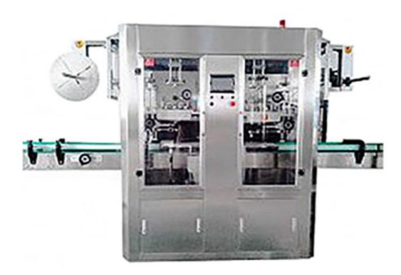
Double-headed shrink label is mainly suitable for the bottle that needs two labels, such as bottle labeling and bottle cap labeling etc. It can save cost and floor area and increase the production efficiency!
