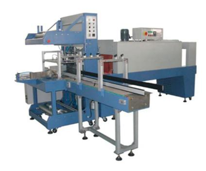
Model BSF-6030XI+BS-6040L is ideal for packaging single and multiple products without tray. The machine can be integrated into a production line to complete the process of product infeed, film wrapping, sealing & cutting, shrinking and cooling automatically. It can handle various packing patterns. For example, the quantity of the bottle to be packed can be 6, 9, 12, 15, 18, 20, 24, etc. per package.
