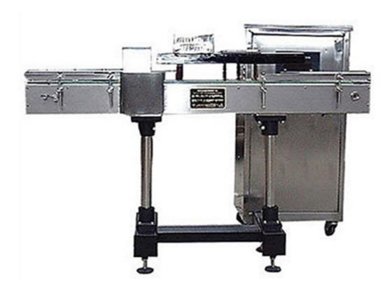
JF-2 is new generation production which adopts electromagnetic induction technical. The machine is economical and easy to operate. It uses widely in food& beverage, Pharmaceuticals and chemical industry etc. This fully automatic sealing machine can seal the mouth of container with aluminum foil at speeds up to 120 cpm.
