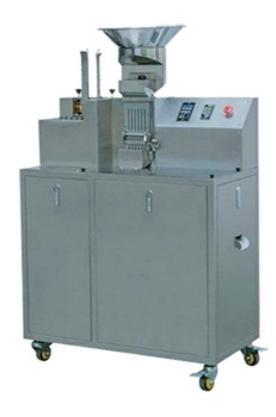
Defects, during medicine production, can cause capsules to be rejected from the capsule filling machine or Blister Machine. Pressing out the capsules from faulty blister cards and separating the capsule from the powder, without cross-contamination, can be accomplished by our machine: The Deblister and Retrieving Machine NQF800.
