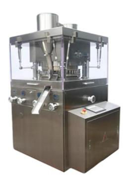
That machine is the latest High Speed Rotary Press Machine in current industry, which development and innovation basis on board and at home technical by our factory; with high speed and high capacity and used to various normal or abnormity tablets pressing; It's the best choice for large Industries of Pharmaceutical, Chemical, Foodstuff, Plastic Electronic producing.
