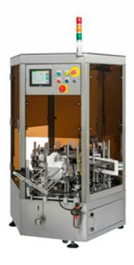
The Vertical Cartoning Machine is popular for pharmaceutical & food industries. It is designed by hexagon shape, which is good for small working space. Any kind of boxes include folding tap, gluing seal or one-touch...etc. all the boxes can be worked basing on customization.
