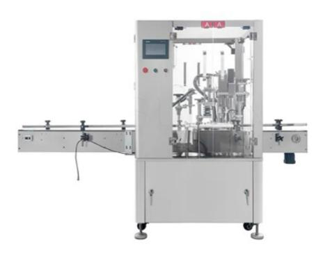
The machine performs automatic filling, automatic capping, and automatic screw capping. It is equipped with PLC control, allowing functions such as no bottle no filling, and no cap no capping, as well as continuous stoppage and rejection of defective products due to missing caps.
