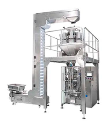
BVL-520 is specially designed for large vertical bags and gusset pillow bags. The bag size, filling volume, etc. can be changed according to customer needs. It is simple and easy to operate. It adopts a servo film pulling system, which operates stably and reliably and avoids film misalignment. Phenomenon, it can package granules such as cereals, sugar, salt, etc., as well as powders such as milk powder and meal replacement powder.
