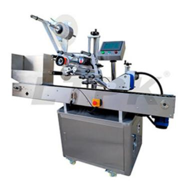
This LTPK LT-330 Automatic Horizontal Round Bottle Labeling machine is suitable for labeling sticker on cylinder which are hard to stand up. The horizontal transmission and labeling can help to improve labeling accuracy and working efficiency. This machine can be equipped with a date coder which can be used to code production date and production number.
