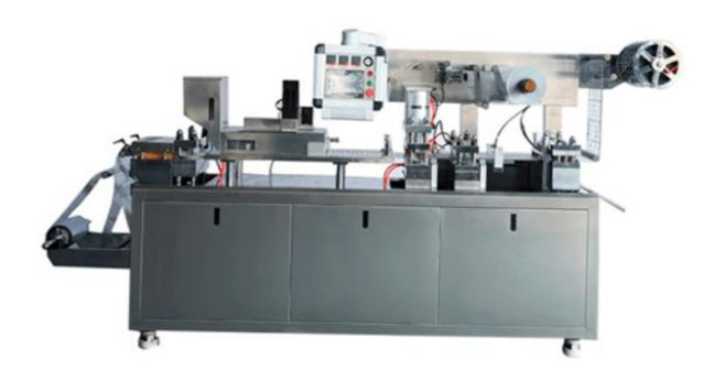
This machine provides packaging of capsules, tablets, pallets and other non-standard objects in blister forms (aluminum-plastic, aluminum-aluminum, aluminum-plastic-aluminum). The machine has small overall dimensions, easily removable replaceable parts, equipped with a control and monitoring system using a programmable logic controller, which ensures the orientation of capsules in accordance with different colors and the receipt of high-quality packaged tablets up to 99.9%.
