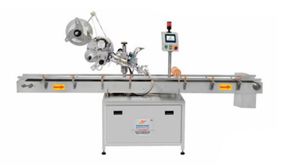
The Automatic Top and Side Sticker Labelling Machine consists of a main structure, product transmission belt with guide adjustment, 2 nos. of label dispensing unit, label pasting by wrapping belt and nylon brush & sponge roller, motors, sensors, electrical panel, PLC & HMI, AC drives & a batch printing unit (OPTIONAL).
